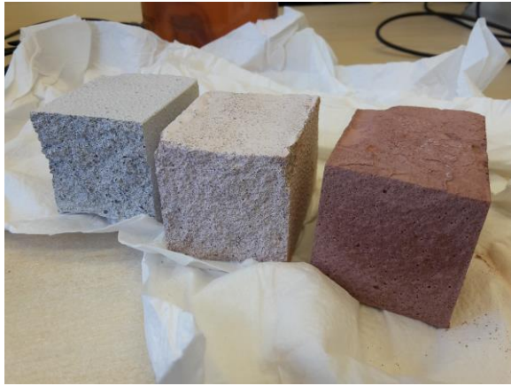
Figure 1. The three building blocks produced in September 2018; f.l.t.r.: Moon Terrae simulant-1, Mars-Jezero simulant 1 and 2. Made with Portland cement. Their strength profiles are comparable to low-grade industrial concrete on Earth.
