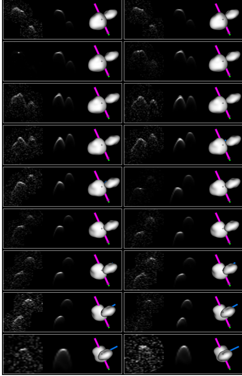
Figure 2. The tiles include three components. On the left is the delay-Doppler data, in the centre is a synthetic delay-Doppler image, and on the right is the plane-of-sky projection of the best-fit model of the asteroid. The green, red, and blue rods mark the asteroid’s inertial axes, and the pink arrow shows direction of the spin-axis. Time progresses from left to right, then top to bottom. The object was observed over two nights on 28 and 29 October 2003.
