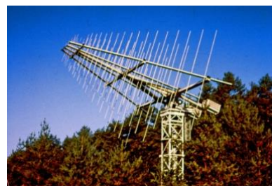
Figure 2: The Nançay Decameter Interferometer included 2 Yagi antenna mounted on mobile booms.
