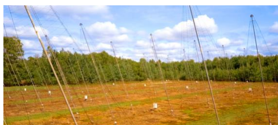
Figure 1: The Nançay Decameter Array is made of 144 helical antennas sensitive to circular polarization.
