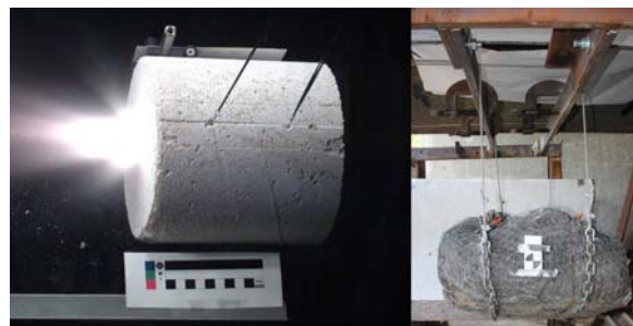
Figure 1: Geometry of typical impact experiment setup for decimeter-scale AVGR targets (left) and meter-scale SwRI targets (right).
