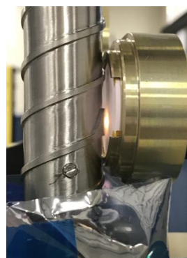
Fig. 2: Ma_MISS light from the zaffire window during tests.
