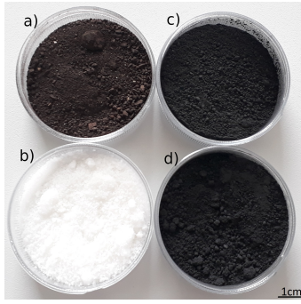
Figure 2: Used organic materials: a) humic acid, b) paraffin, c) graphite, 10,75 \mu\text{m} in radius, d) graphite, 4,15 \mu\text{m} in radius.
