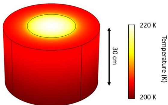
Figure 1: Example of the thermal model for a CoPhyLab sample heated from above by a solar simulator and cooled by thermal radiation
