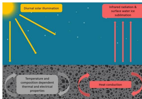
Figure 1: Schematic representation of the thermal model used for the CoPhyLab samples.
