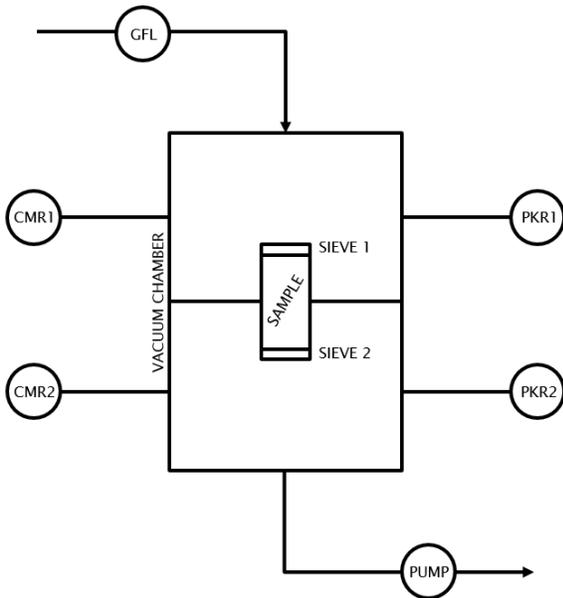
Figure 1: Scheme of the Gas Flow experiment
