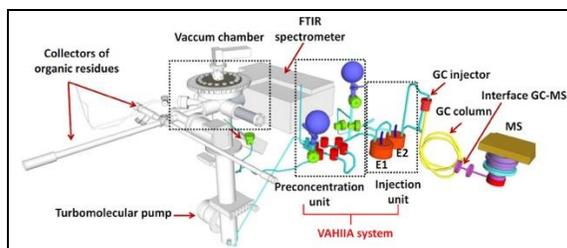
Figure 1: Schematic representation of AHIIA high vacuum chamber experiment developed in PIIM laboratory.
