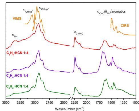
Figure 3: Comparison of  $\text{C}_6\text{H}_6:\text{HCN}$  (1:4; 1:1; 4:1 mixing ratios) photopolymers infrared spectra recorded at 300K with VIMS/CIRS data.
