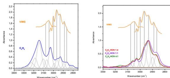
Figure 2: Comparison of pure  $\text{C}_6\text{H}_6/\text{C}_6\text{H}_6:\text{HCN}$  1:4; 1:1; 4:1 mixing ratios) photopolymers deconvoluted infrared spectra recorded at 300K with VIMS data.
