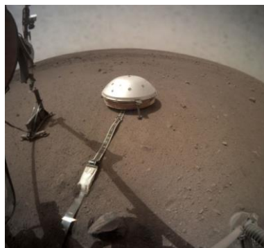
Figure 1: The InSight Seismometer SEIS deployed on the surface of Mars under the Wind and Thermal Shield.
