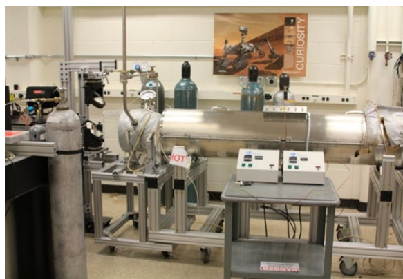
Figure 3. The 2 m long, 110 mm diameter Venus chamber used for sample analysis at >92 atm of CO 2 at >465°C.
