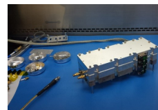
Figure 3. Flight Model of the transponder while mounting the PCBs (Printed Circuit Board).
