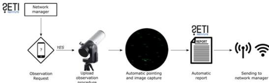
Figure 3: Campaign Mode schematic as designed by Unistellar. In this case, the flyby of the 650m NEA 2014 JO25 was observed in April 2017.
