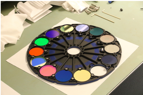
Figure 1: CometCam filterwheel in the clean room at LCO headquarters. The ESA comet filters are the six thicker filters towards the top right of the image. Filters are 50mm diameter and the filterwheel is 300mm across.
