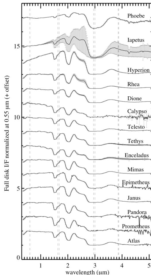
Figure 1: VIS-NIR disk-integrated average reflectance spectra ( $\pm 1\sigma$ ) of the saturnian icy satellites. Spectra are normalized to 1 at 0.55  $\mu\text{m}$  and stack with an offset for clarity. The satellites are sorted according to their distance from Saturn. Vertical lines indicate the spectral position of the instrumental order sorting filters.
