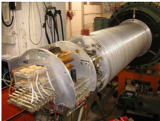
Figure 1 : Acceleration path and dust source of the 2 MV Van-de-Graaff dust accelerator.
