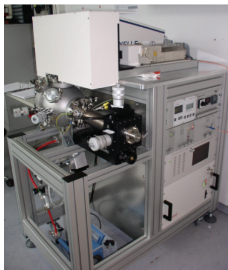
Figure 1: LIBS system with planetary simulation chamber.
