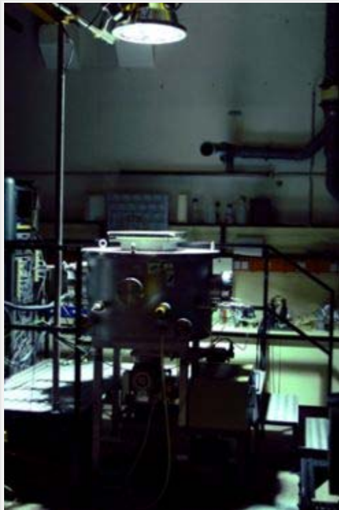
Figure 1: Test chamber used for an EVT with a light source SOL 2000 for the solar UV simulation
