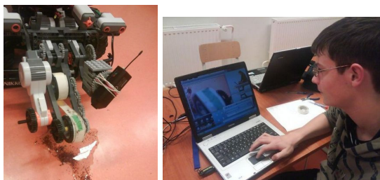
Fig. 4. Control room student observes on the screen the measured color, and he can compare the measured value with the standard color set of the pH-values. (Languages: Labview; on the terrestrial control computer, MSWLogo; for the transliteration of color to pH-value.)
