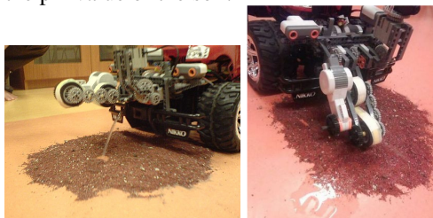
Fig. 3. Pouring water, the indicator arm touch the soil. Indicator ribbon arm rolls the ribbon. Husar moves backward to prepare observation of the rolled indicator surface, which holds the information about the pH of the soil. The result of the experiment on the indicator ribbon is transferred by the camera.
