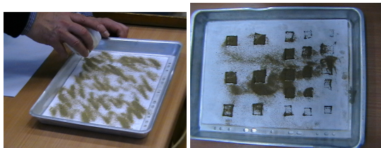
Fig. 1. Magnetic experiment in the lab. dispersing the mixture on the magnetic carpet (here white sheet) the magnetic component of the dust adheres above the magnetic squares.
