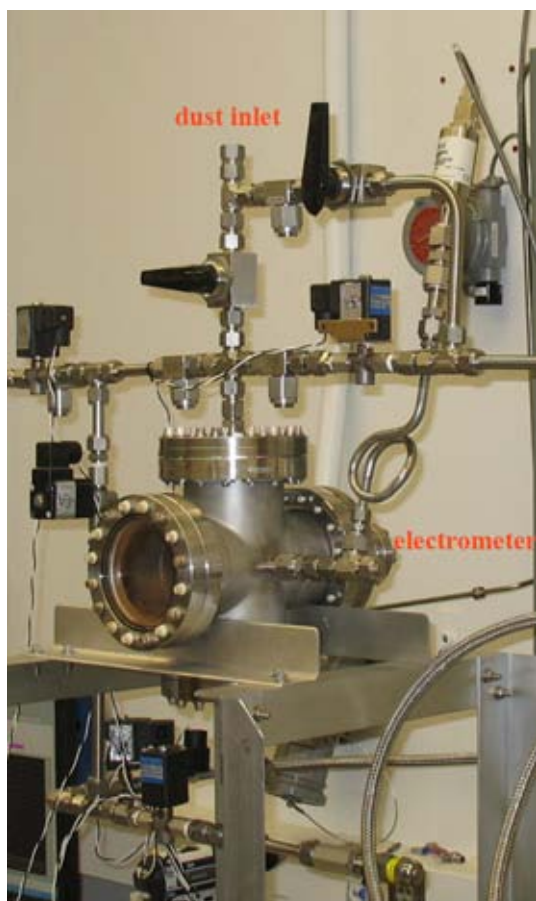
Figure 2. The experimental dust circulation chamber, with the dust inlet on the top. The electrometer is attached to the back. Gas is pulsed in through the bottom.
