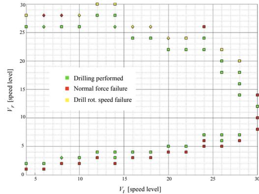
Figure 3: Gasbeton working zone;  $0^\circ$  surface inclination, torque levels 4 and 2 for the drill translation and rotation motors.
