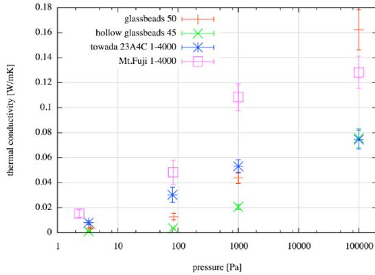
Figure 1: Thermal conductivity as a function of pressure. The pairs of glass beads and natural products have the same size respectively. The samples represented in blue and green plots have the same bulk porosity.
