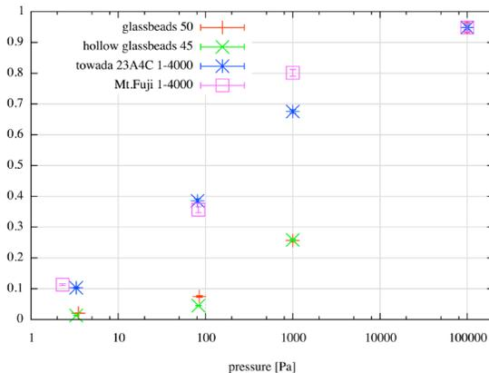
Figure 2: Normalized thermal conductivity under low pressures. The thermal conductivity under atmospheric pressure (1013 hPa) is standard. The pairs of glass beads and natural products have the same size respectively. The samples represented in blue and green plots have the same bulk porosity.
