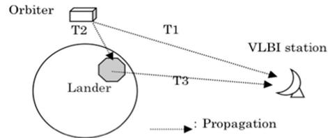
Figure 3: The principle of inverse VLBI in the case of an orbiter and a lander.
