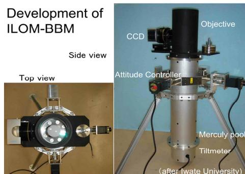
Figure 1: BBM of ILOM model. Attitude control system is attached to the outside of the telescope tube. Optical tests with CCD and light sources are performed using this model.
