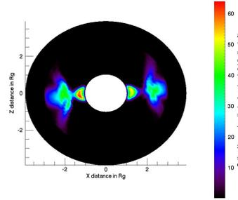
Fig 2: Oxygen ions trapped at 25KeV
