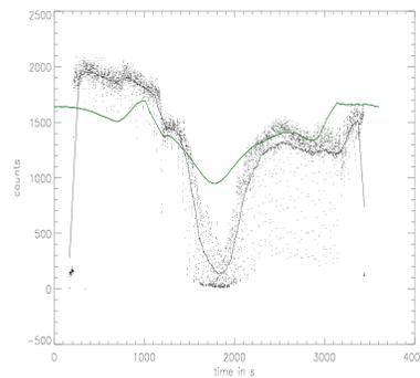
Fig 3: Electron simulated (green) and observed (black and dot) counts for chanel F2 of EPD instruments during the G2 flyby.
