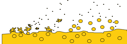
Figure: 1 Dust aggregates being entrained and liberating dust below the saltation threshold
