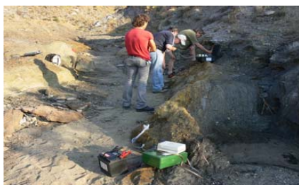
Figure 1- Mössbauer, Raman and LIBS instruments displayed at an outcrop with clay minerals covered by jarosite and oxi-hydroxide deposits.
