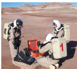
Figure 3: In-Sim deployment of the Terra X-Ray Diffraction Analyzer [4].
