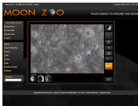
Figure 1: The Moon Zoo interface facilitates citizen scientists annotating LRO images with the locations of various geologic features, as well as the locations of spacecraft.
