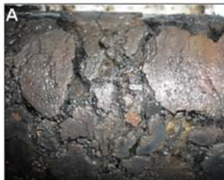
Fig. 1: Lateral view of a core obtained at depth of 60-80 cm, with relatively high water content and big ice crystals.
