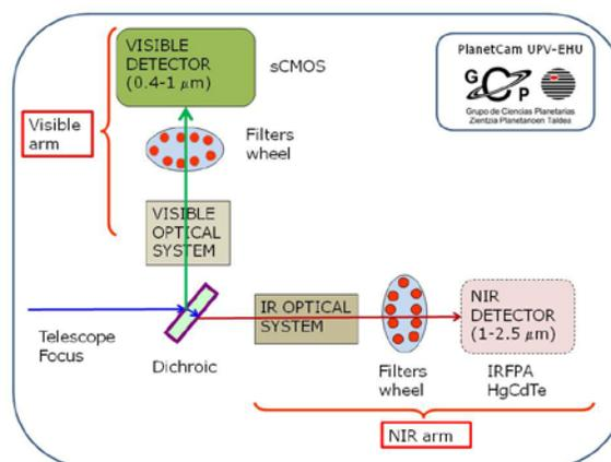
Figure 1: Scheme of PlanetCam UPV/EHU
