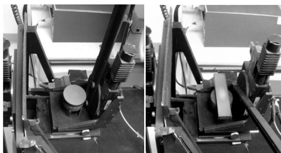
Figure 1: BUG Experimental Setup. (left) Full bidirectional reflectance measurements are performed using 28g of lunar soil in a circular dish at incidence angles ranging from 0^\circ to 60^\circ . (right) By placing the same soil sample in an elongated rectangular trough, bidirectional reflectance measurements are performed inside and perpendicular to the principal plane at incidence angles of 70^\circ and 75^\circ
