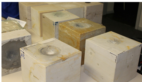
Fig. 1: A selection of experimental impact craters formed in 20 cm edge-length sandstone targets at impact velocities of ~5 km/s. Experiments using tuff and quartzite targets will be compared to these results.
