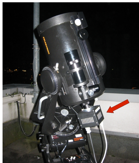
Figure 1: The SPOSH camera head mounted onto the telescope (red arrow)
