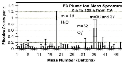
Figure 1: Mass spectrum measured by the Cassini INMS during the E3 Enceladus encounter. Effective count rate versus mass number (in atomic mass units). From Cravens et al. (2009) [1].
