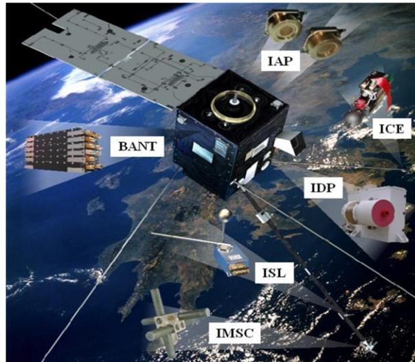
Figure 1: The schematic view of the DEMETER satellite and its instrumentation.
