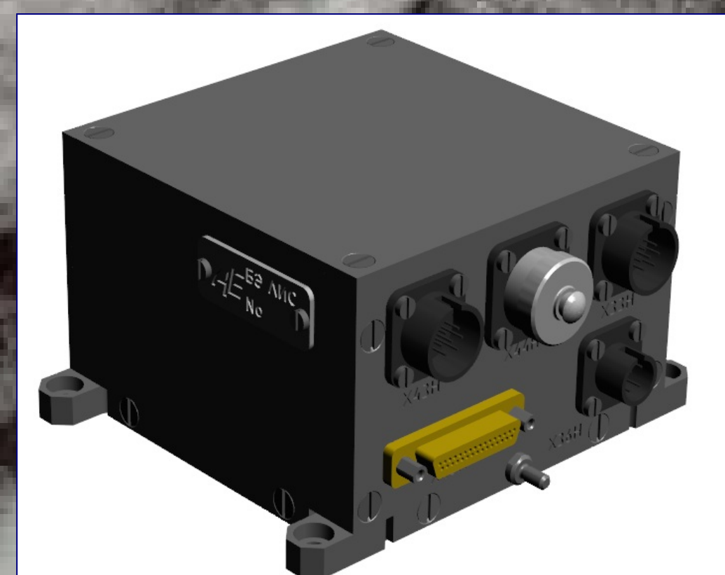
Fig. 2. Electronics box of the spectrometer
