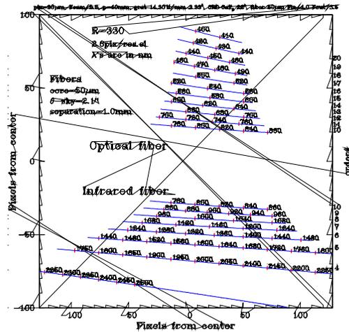
Figure 1: Positioning of the spectrum on the VNIR 256 x 256 pixels detector.
