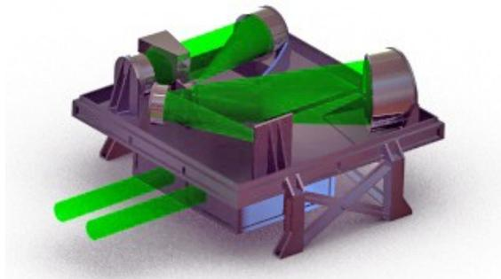
Figure 2. Opto-mechanical layout of the module
