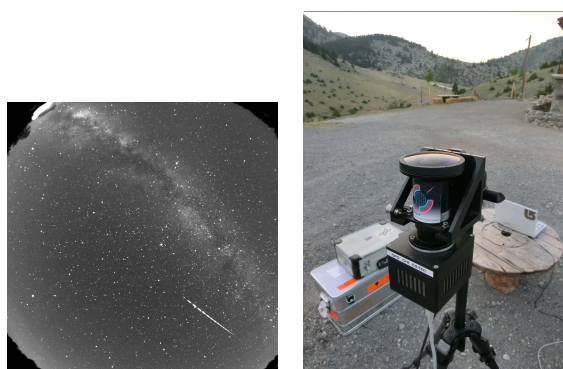
Figure 1: A long Perseid meteor captured by the SPOSH camera operated in Mt. Parnon during the last 2012 observing campaign in Greece (left). The camera breadboard mounted on a tripod in Mt. Mainalon.
