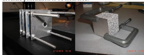
Fig. 2 Left: four plate Whipple target (post-impact). Right: Aluminium foam sandwich target (pre-impact). Plates = 35 mm 2 .
