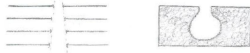
Fig. 3 Cross-sectional sketch of penetration path. Left: Conical in Whipple plates. Right: Bulbous cavity formed in aluminium foam.
