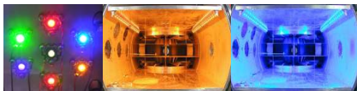
Figure 3 section of the multi wavelength LED light source (left) and wind tunnel tests section using different lighting settings (center/right).
