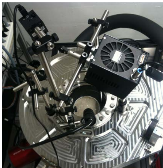
Figure 1: Picture of the simulation chamber showing a sample of clay/sodium chloride mixture through the upper window and cameras and illumination fibres fixed around the window.
