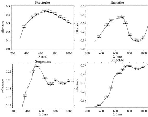
Figure 1: Absolute spectrum of selected silicates as seen by OSIRIS NAC filters listed in Table 1. Solid lines are laboratory data of corresponding mineral, while dots are sampled spectra. Bandwidths are indicated with horizontal bars.
