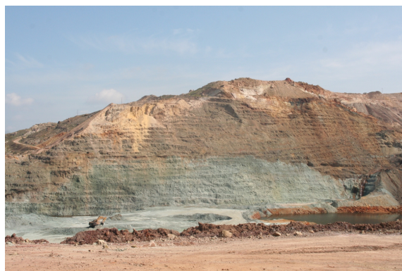
Figure 1: View of the SW Skouriotissa pit with the brown gossan at the top and the green quartz-chlorite pillow basalt formation at the bottom. Note the mechanical stripper bottom left for scale.
