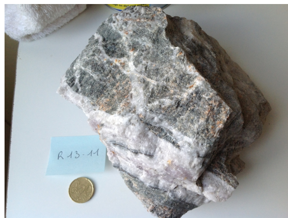
Figure 1: Photography of hydrothermal veins in a massive granular rock. Note the breccias structure and locally the geodic aspect of the vein filling.
