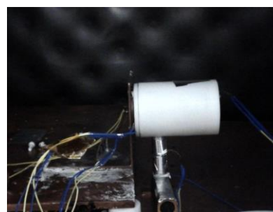
Figure 1. Cylindrical case and beaker containing the dicarboxylic acid.
