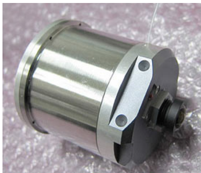
Figure 3: A photograph of IKAROS DCAM1,2. Body diameter is approx. 60 mm.
