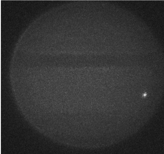
Figure 1: detection image generated by DeTeCt software (image with maximum value minus mean value for each aligned pixel) from an acquisition from Christopher Go on June 3rd 2010 with a ream detected impact
