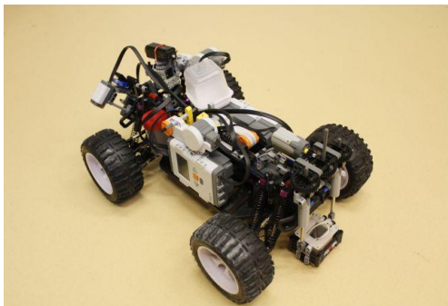
Fig. 1. The Husar-5 rover with the Carbonate experiment when coil of the magnetic experiment is in lowered position.
