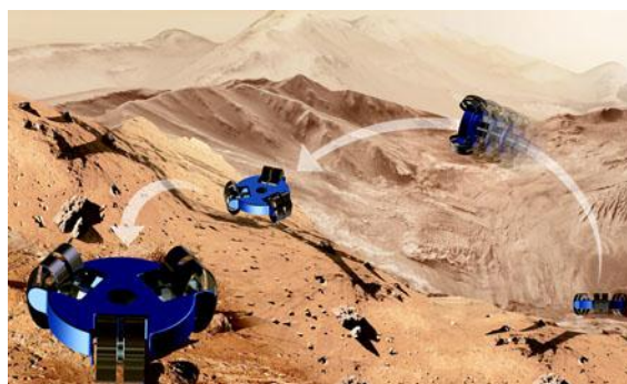
Figure 1. The Highland Terrain Hopper is a light and symmetric jumping robot developed by Astronika Ltd. and the Polish Space Research Centre (here jumping within a Valles Marineris-type landscape).
