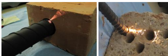
Figure 2: Two different moments of the Ma_Miss tests during the drilling. The light beam comes out
